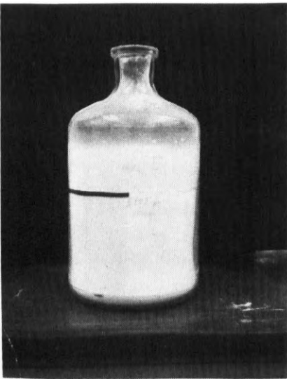
Fig. 5. Six liters Borax TM powder in a jar with two liters of Silanox TM poured on its surface.
